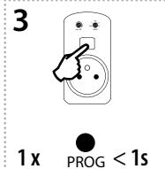
Press of programming button on socket RFDSC-71 shorter than 1 second will finish programming mode. The LED lights up according to the pre-set memory function.
