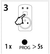
Press of programming button longer then 5 seconds, will activate socket into timing mode. LED flashes 2x in each 1s interval. After releasing the button, the time of the sunset function begins to count down (period of complete dimming of the light).
