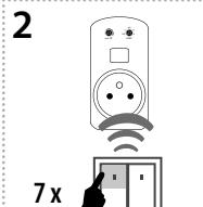
Seven presses of your selected button on the RF transmitter assigns the function ON/OFF (must be a lapse of 1s between individual presses).
