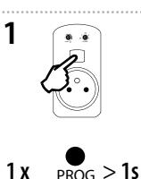
Press of programming button on socket RFDSC-71 for 1 second will activate socket RFDSC-71 into programming mode. LED is flashing in 1s interval.
