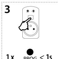
Press of programming button on actuator RFDSC-71 shorter than 1 second will finish programming mode. The LED lights up according to the pre-set memory function.
