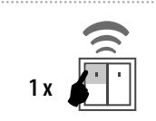
After pressing the programmed button, the light begins to dim in the programmed time interval in a range of 2 seconds to 30 minutes.
