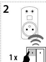
A press of your selected button on the RF transmitter assigns the function light scene 1.
