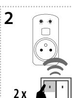
Two presses of your selected button on the RF transmitter assigns the function light scene 2 (must be a lapse of 1s between individual presses).
