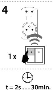
After the desired time has elapsed, the timing mode ends by pressing the button on the RF transmitter, to which the sunset function is assigned. This stores the set time interval into the socket memory.
