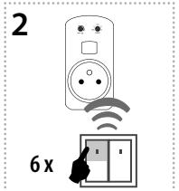
Assignment of the sunset function is performed by six presses of the selected button on the RF transmitter (must be a lapse of 1s between individual presses).
