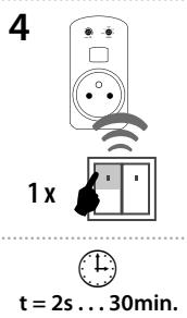
After the desired time has elapsed, the timing mode ends by pressing the button on the RF transmitter, to which the sunrise function is assigned. This stores the set time interval into the socket memory.
