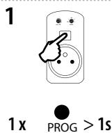
Press of programming button on socket RFDSC-71 for 1 second will activate socket RFDSC-71 into programming mode. LED is flashing in 1s interval.
