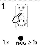
Press of programming button on socket RFDSC-71 for 1 second will activate socket RFDSC-71 into programming mode. LED is flashing in 1s interval.
