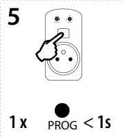
Press of programming button on socket RFDSC-71 shorter then 1 second will finish programming mode. The LED lights up according to the pre-set memory function.
