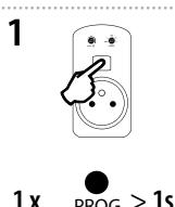
Press of programming button on actuator RFDSC-71 for 1 second will activate actuator RFDSC-71 into programming mode. LED is flashing in 1s interval.
