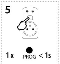
Press of programming button on socket RFDSC-71 shorter then 1 second will finish programming mode. The LED lights up according to the pre-set memory function.
