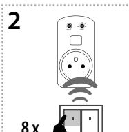
Eight presses of selected button on the RF transmitter assigns the function OFF (must be a lapse of 1s between individual presses).
