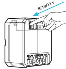
If you want to clear the memory of the whole device (unpair all buttons or delete all channels at once, press the PROG button on the device for 8/10/11 s according to the type of device (see. **Tab 1**). Clearing the memory of the entire device. The device remains in pairing mode.
